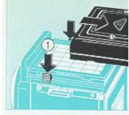
To lift the focusing screen: take hold of the two sides of the frame, pull backwards slightly and lift (2) Close by pushing downward.
