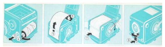
To open camera: turn the safety back lock clip at the tripod socket (I), lift back lock lever (a) and pull back open.
