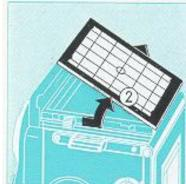
**Adjusting the ever-ready case** to the larger diameter of the Rolleikin counter knob: remove leather insert at the left side after bending the metal retaining clips upward.
