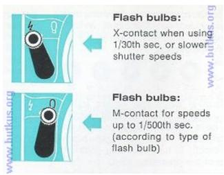
The correct exposure depends on the light output of the flash and the distance between flash and subject. Therefore, it cannot be determined with an exposure meter. Exact data regarding choice of proper contact, exposure time and diaphragm may be gathered from the instructions furnished by the lamp manufacturers....
